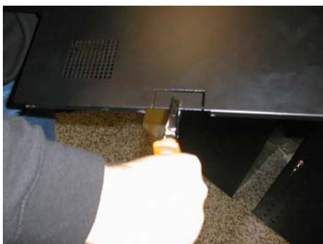
Cut the rear wall to make a hole for Damian Piccola to connect the communication cable. Install again the rear wall of the XS H - XS H/LIONESS vending machine.
