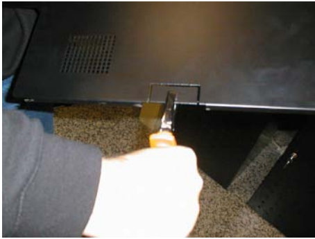
Cut the rear wall to make a hole for Damian Piccola to connect the communication cable. Install again the rear wall of the XM vending machine.
