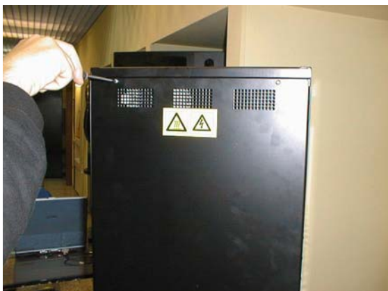
Disassemble the rear wall of the XS H - XS H/LIONESS machine unscrewing the fixing screws.
