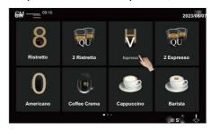
Step2: Drink under processing, click the button"^", Pop-up window of parameter adjustment, click of"-4" to temporarily adjust the amount; (Available only in adjustable mode)
