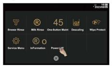
Step 3: The screen pop-up prompts. Are you "power off', click "Yes" machine turns to power off mode, click "No" to cancel this operation, the screen is off but light is still on (press the screen more than 3 seconds to wake up the machine)
